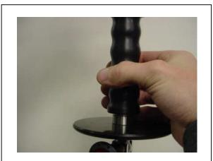
If you relieve the carpus and give small, precise movements with your fingertips the hoist will move with a low and controlled speed, this grip is good when handling fragile goods, fitting the lift object when assembly, fixtures e.t.c.
