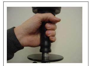
Using the whole hand gives big movements and therefore a high lifting speed of the hoist, this grip can be used when handling not fragile goods.
